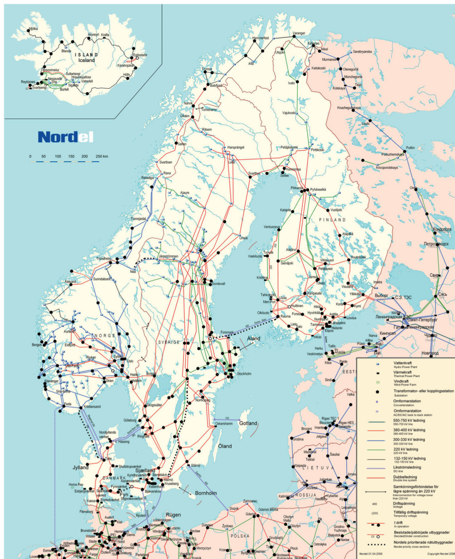
Figure 2.1 The transmission grid in the Nordic countries.
